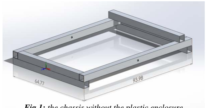
Fig 1: the chassis without the plastic enclosure coverings. Dimensions are in centimeters
