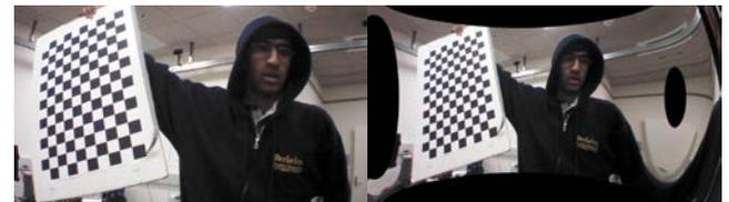
(a) original calibration target (b) corrected image
