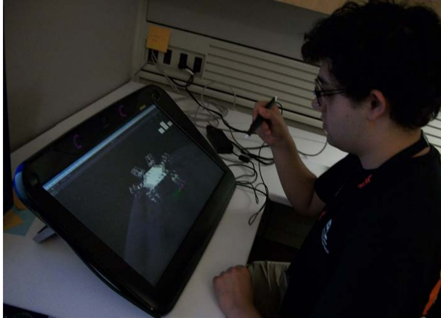
Figure 6: User positioning the end effector with the device as part of the drilling application. Notice the stereoscopic rendering and stylus usage.
