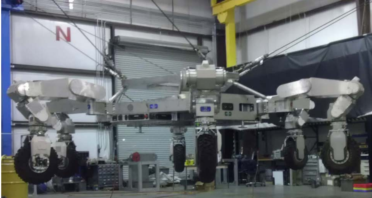
Figure 1: ATHLETE in the Microgravity Testbed, where it is being repurposed for a possible future asteroid exploration mission. (Tri-ATHLETE version with 6 DoF limb configuration)
