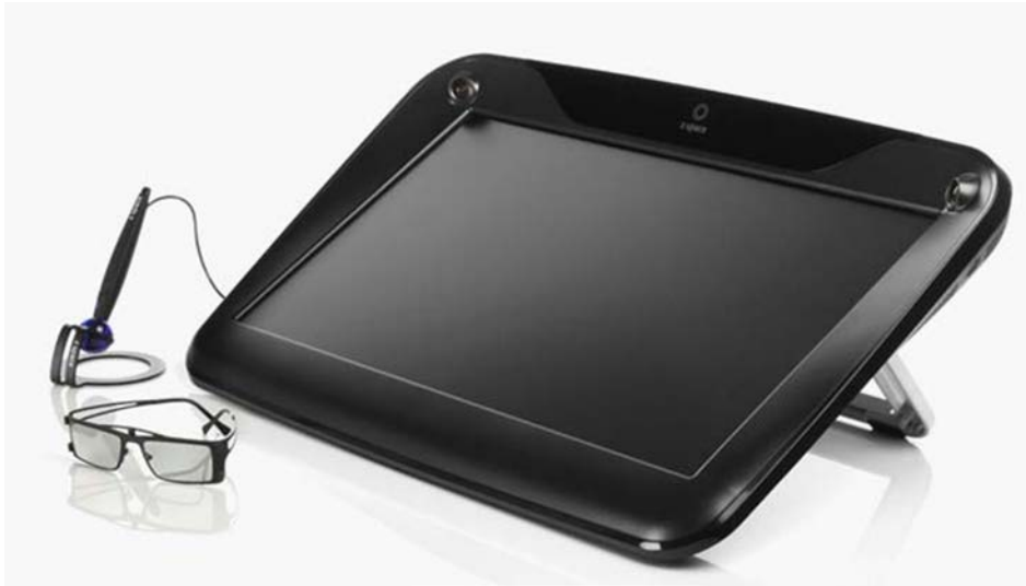
Figure 3: The zSpace device, including the 3D display with built-in infrared projectors and infrared tracking cameras as well as the stylus and passive polarized glasses.
